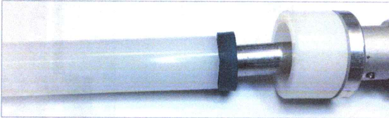
FIGURE 4 – PUSH TUBE, used to push LIP SEAL onto piston rod and into compression ring into PISTON ROD GUIDE BUSHING.
