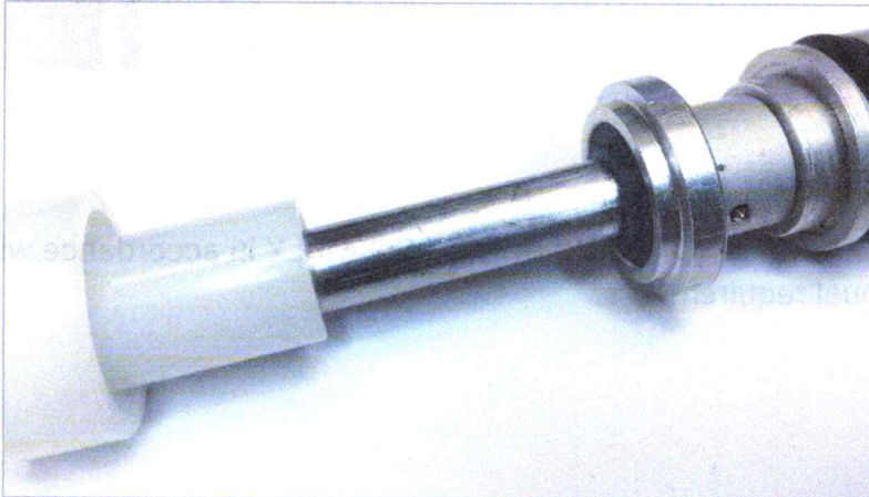
FIGURE 5 – Once LIP SEAL is fully inserted into PISTON ROD GUIDE BUSHING, remove all tooling.
