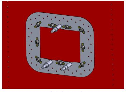
**STEP 3**: Remove doubler, debur drilled holes, and Cleco the AOA Probe Mounting Template (AOA-4203) using the 3 reference holes. Scribe/mark around the edge of the AOA mounting
