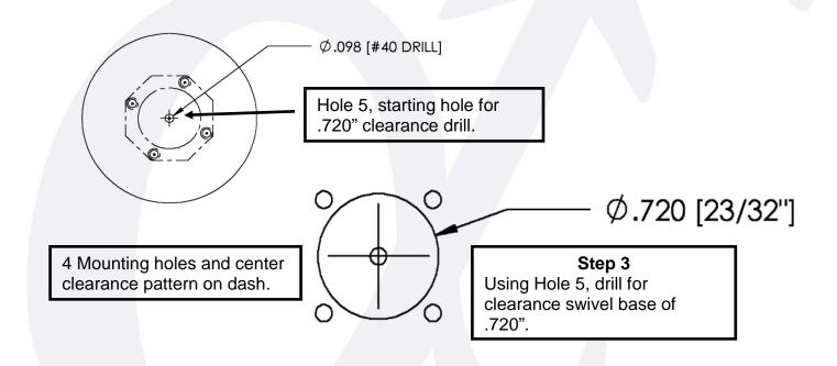
Once the 4 outer holes are located and drilled, re-drill with a # 32 (.116") clearance for the 4-40 mounting screws.
