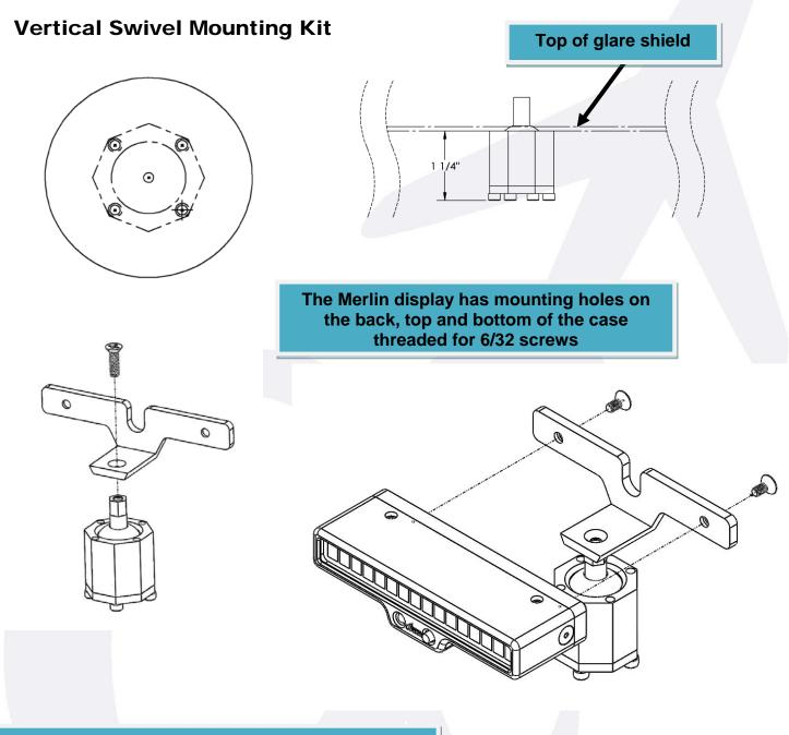
The swivel kit is mounted from under the glare shield and the shaft allows the L bracket to be mounted solidly with the provided screw
