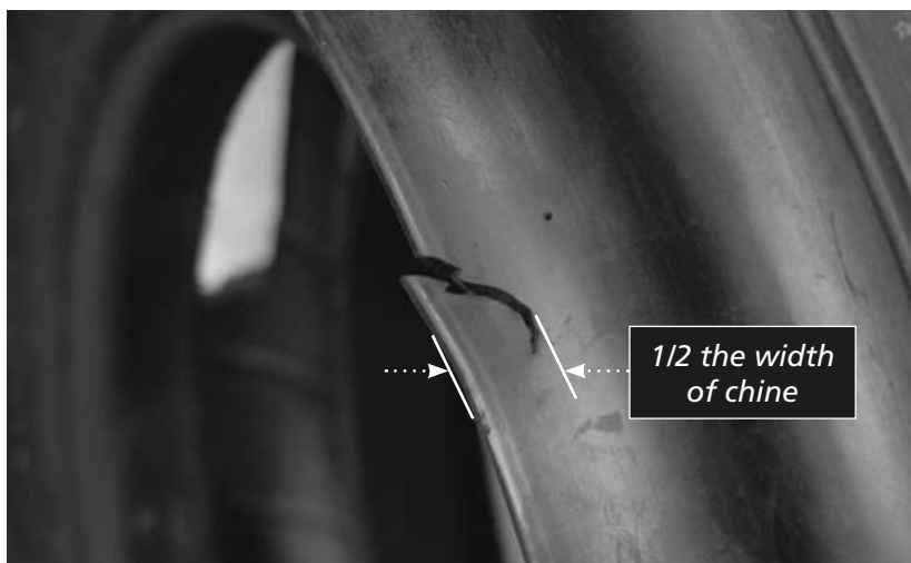
Figure 528. Damage to Chine Tire
