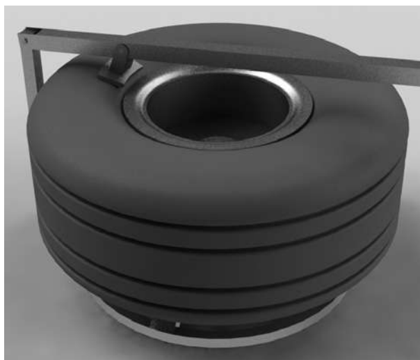
Figure 602. Lever Arm Bead Breaker
