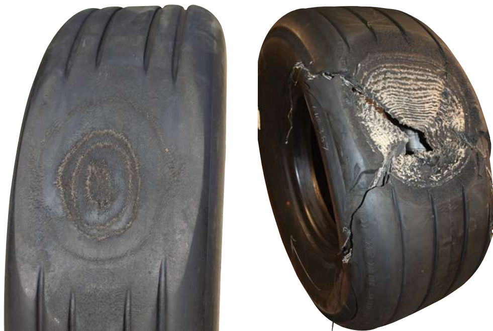
Exposed Reinforcing Plies
