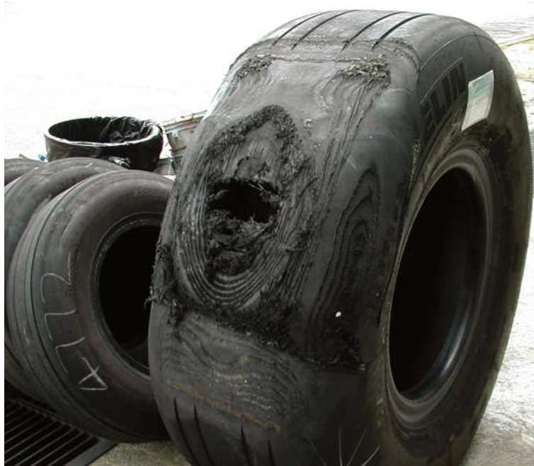
Figure 509. Flat Spot Resulting in Tire Rupture - Radial
