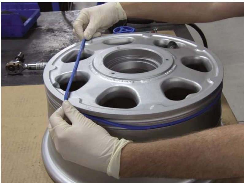
Figure 404. Installation of O-Ring on Inner Wheel Half
