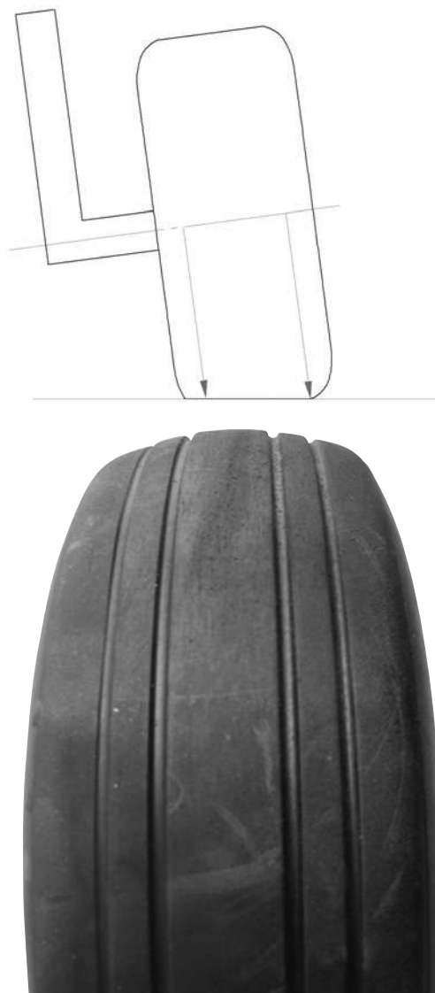
Figure 511. Camber Angle – Negative Camber
