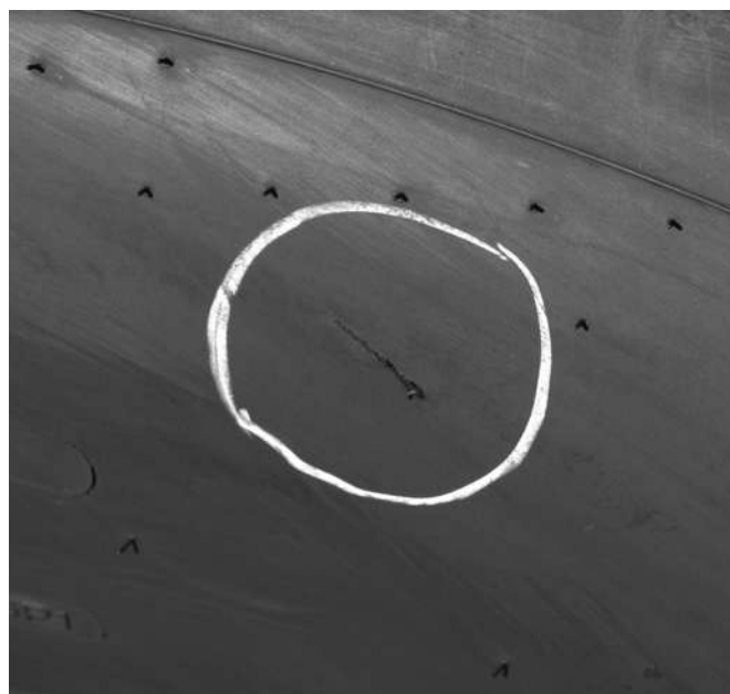
Figure 302. Damage From Contact With Sharp Object - Serviceable
