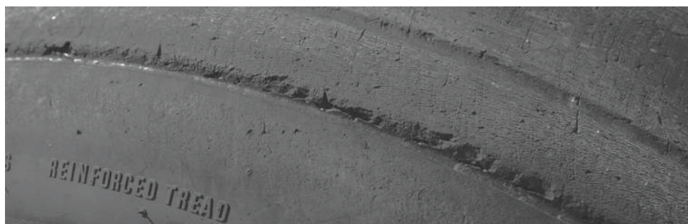
Figure 518. Groove Edge Chunking
