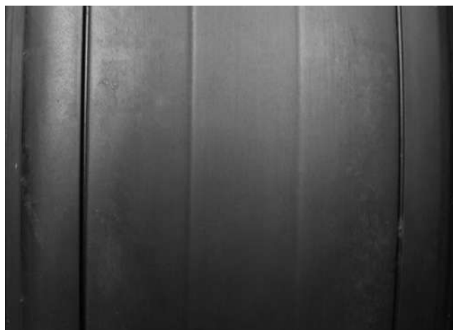
Figure 504. Normal Removal Wear
