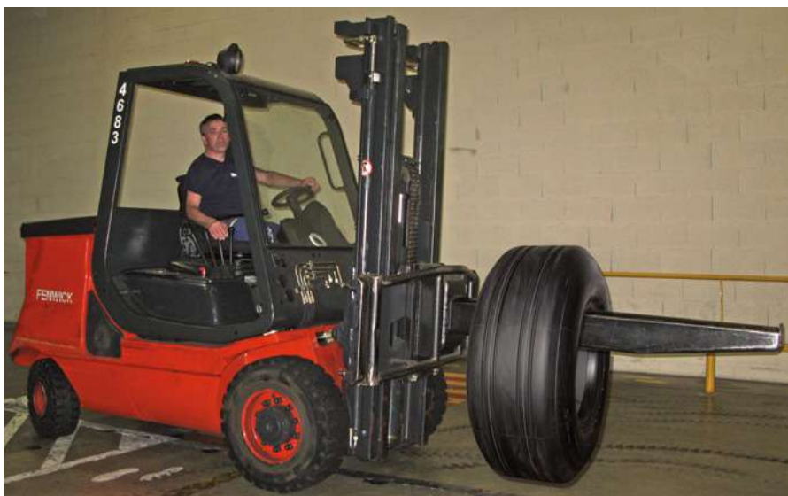
Figure 301. Damage From Lift Truck Forks (Left). Tires Can Be Lifted Through the Center (Right).
