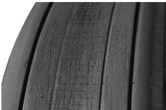
Figure 516. Aggressive Wear from Heavy Braking
