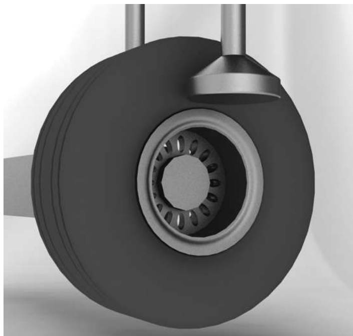
Figure 607. Conical Roller Bead Breaker – Two Rollers
