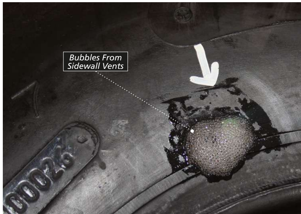
Figure 107. Appearance of Bubbles From Tire Vents
