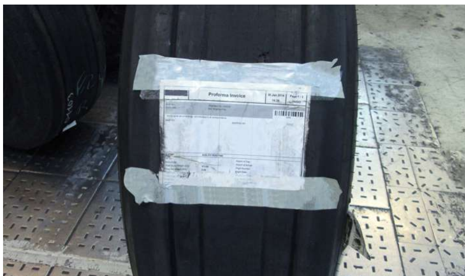
Figure 613. Recommended Placement of Adhesive Labels on Tires
