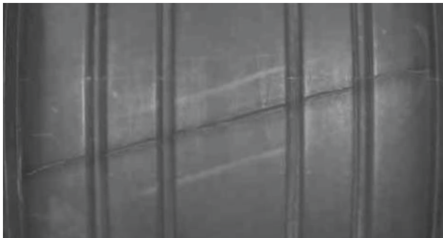
Figure 522. Open Tread Splice
