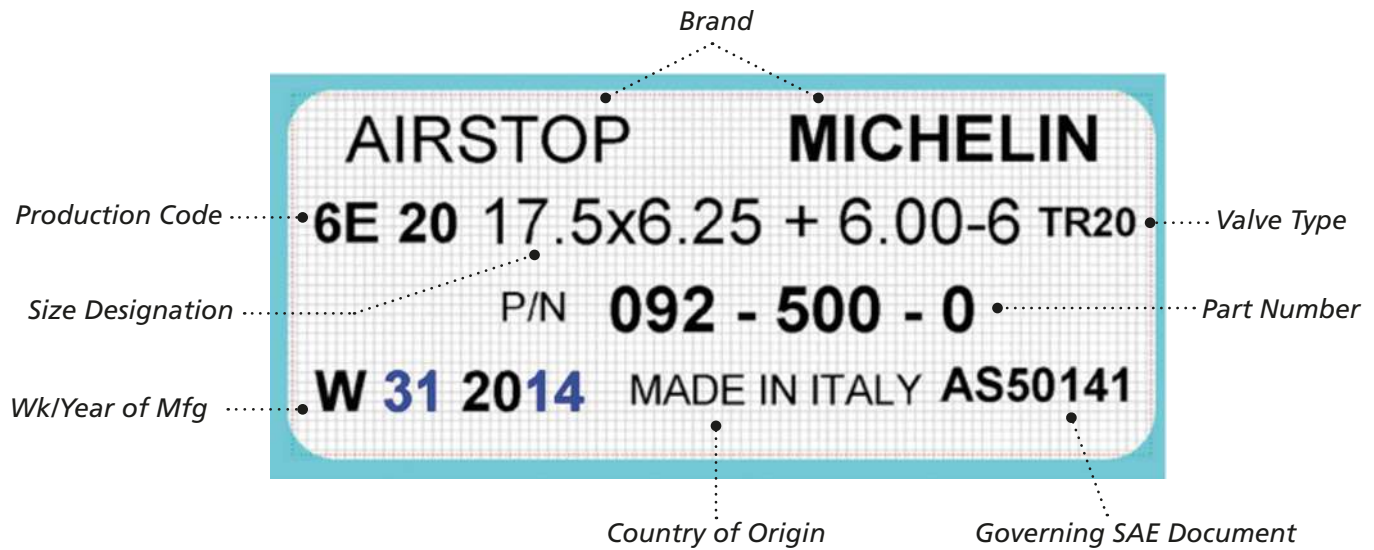
Figure 207. Typical Aircraft Tube Markings
