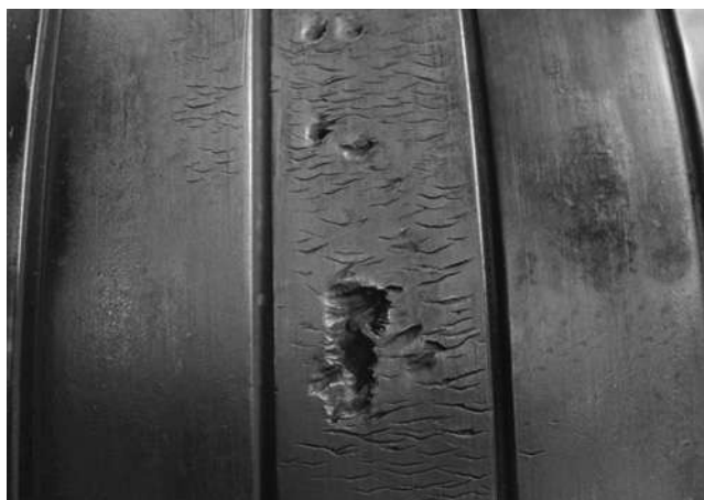
Figure 515. Chevron Cutting – Exposed Ply
