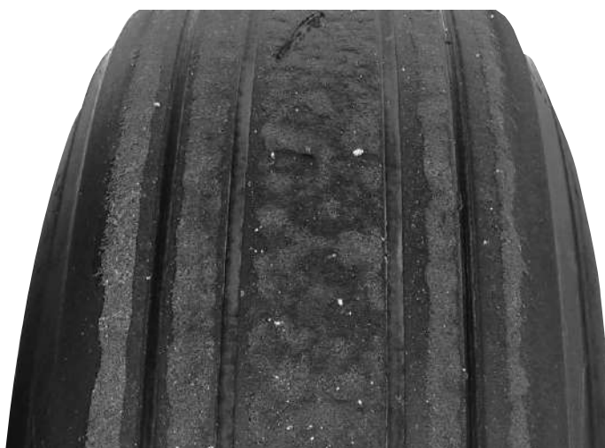
Figure 533. Contamination From Hydrocarbons
