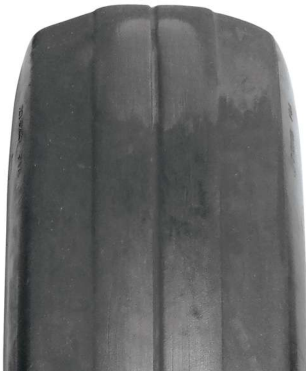
Figure 507. Shoulder Wear due to Underinflation
