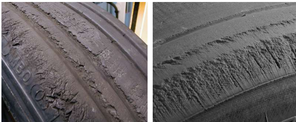
Figure 530. Lateral Scuffing, High Speed Turns, Pivot Turns
