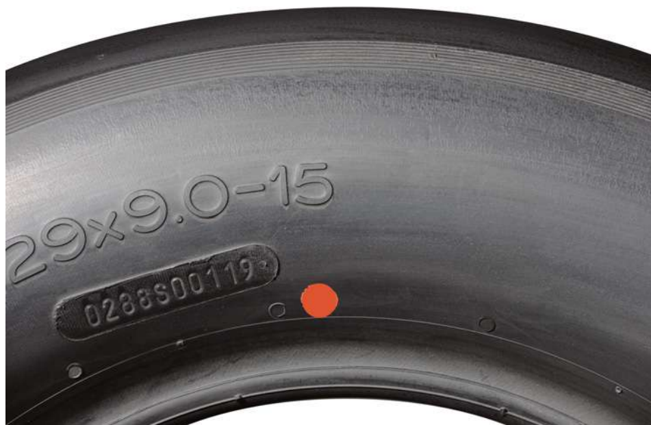
Figure 405. Tire's Red Balance Mark
