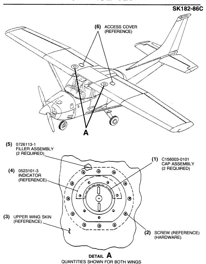
Figure 1. Fuel Cap and Adapter Modification
