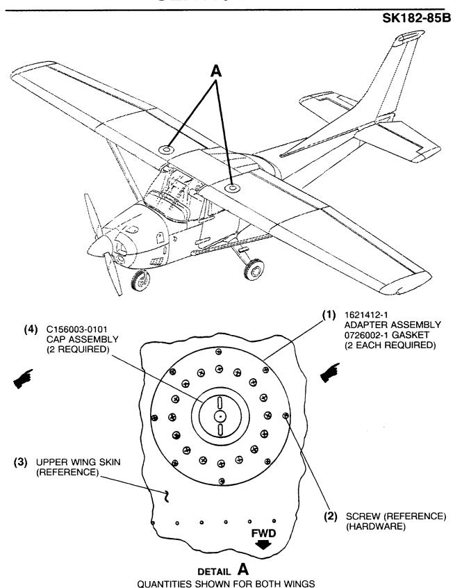
Figure 1. Fuel Cap and Adapter Modification
