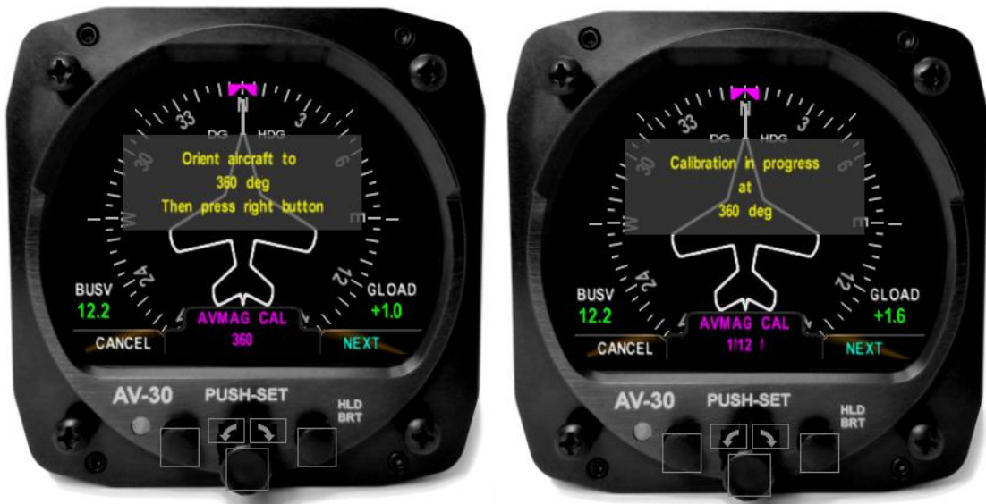
Figure 28 – AVMAG CAL In-Progress
