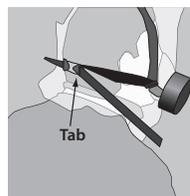
1. First lift the tab (protruding end) of one connecting buckle with one hand and with your other hand pull the elastic strap towards the front.
