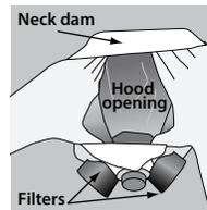
3. With the nose cup and filters facing down towards your body, stretch the hood opening out by placing your fingers in the neck dam with your thumbs spread wide and the back of your hands facing each other.
