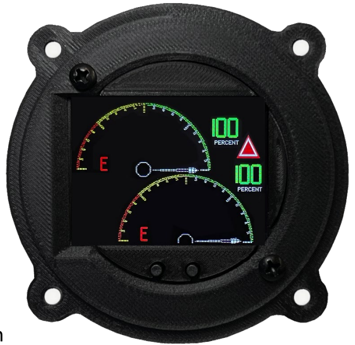
Fuel Gauge showing two tanks in analog and digital formats. Warning symbol also displayed.
