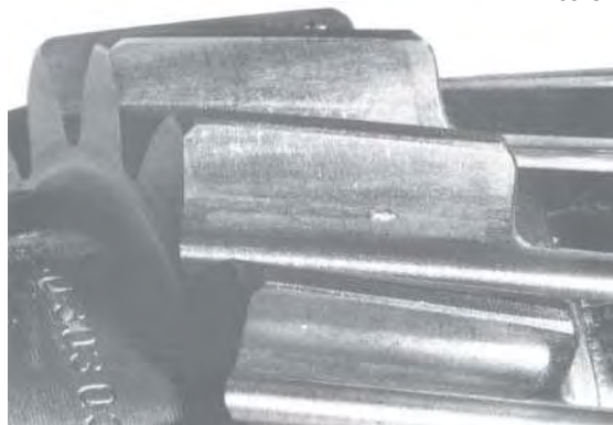
Pitting formation at the foot of spur toothing
