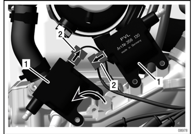
1. Double ignition coils 2. Ignition coil connector (coil 1, coil 2, coil 3, coil 4)
