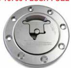
The unvented flush fuel cap operates with a lift and turn lever. This cap has a 3" opening for easy refueling. Cap & adapter ring are anodized "clear" for corrosion resistance. Cap is fastened to adapter ring with safety chain. Made in the U.S.A.
