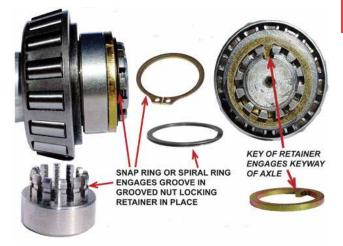
True-Lock aviation fastener systems reduce premature wear on your wheel-end assembly parts (brakes, bearings, axles, including tires and wheels). The True-Lock system eliminates the conventional axle nut system's inherent inferior torque setting characteristics imposed by the castle nut and cotter pin (end-play).
