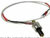
P-Leads are a critical part of the ignition system and their good condition is vital to safety and airworthiness. P-leads are often overlooked and seldom replaced because replacement p-leads are not available from the aircraft manufacturer and materials to fabricate new p-leads are not commonly available. Because most leads are shielded, mechanics do not
