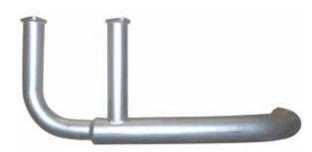
Piper PA-11 Style Exhaust Stack with Starter (Left). Experimental Use Only. Longer down pipes to clear starter, Left Hand. Can be used on Piper J-3, but some modifications of cowling may be necessary. Starter Left......P/N 05-12465 Starter Right ......P/N 05-12466
