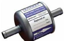
The AA101-524009-0163 is approved on the Beechcraft B200, B200C, B200CT, B200CT and B200GT. This filter is manufactured using a stainless steel housing and .3 micron media. Designed to withstand the toughest environments, the AA101-524009-0163 rudder boost filter continues the long line of dependable and pilot preferred Tempest
