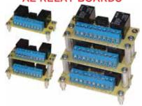
AE Relay Boards - Better than the Competition. These relay contacts are protected against inductive sparking generated from relays switching inductive loads such as motors and solenoids. The relay coils are also protected. This prohibits the relays from early failure. This also protects the switch contacts that drive the relay coils from failure.
