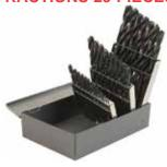
Drill Bit Set Fractions 1/16-1/2 High Speed. Tired of always looking for that drill bit you desperately need? Now you can have all of them right at you fingertips. All Index boxes are the highest quality made. Made in the U.S.A. 29 total pieces plus index box. 135 degree split point (**Note**: Bits smaller than .0625 have no split point) P/N 12-05115
