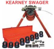
This portable, hand-operated roll type swaging machine will swage MS type terminals onto galvanized and stainless steel cables from 1/16" diameter up to and including 3/16" diameter. Includes machine, a full set of roll dies, terminal gauges and feed guide adapters & instructions in a steel carrying case. Wt. 95 lbs. New manufacture. All replacement parts available.
