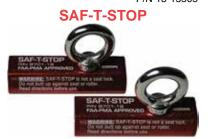
Saf-T-Stop is an auxiliary seat stop mechanism approved by the FAA for use with Cessna seat track A.D. #87-20-03. Installs easily, sliding over seat track. Approved for: Cessna 150, 152, 170, 170B, 172, R172, 175, 180, 182, 185, 190, 205, 206, 207, 210, 303, 337. Not a seat lock, Saf-T-Stop is designed to restrict rearward motion if the seat lock fails. P/N 13-18510/pr
